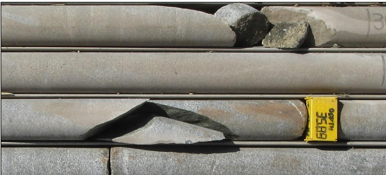
Figure 9.11 – Example of typical joint surface in norite showing smooth, undulating surface
