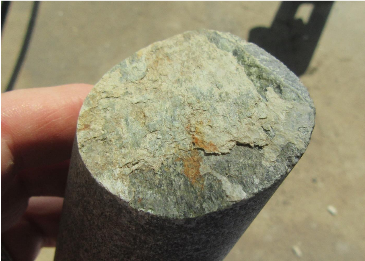
Figure 9.10 – Example of typical joint surface in pyroxenite with slickensided infill
