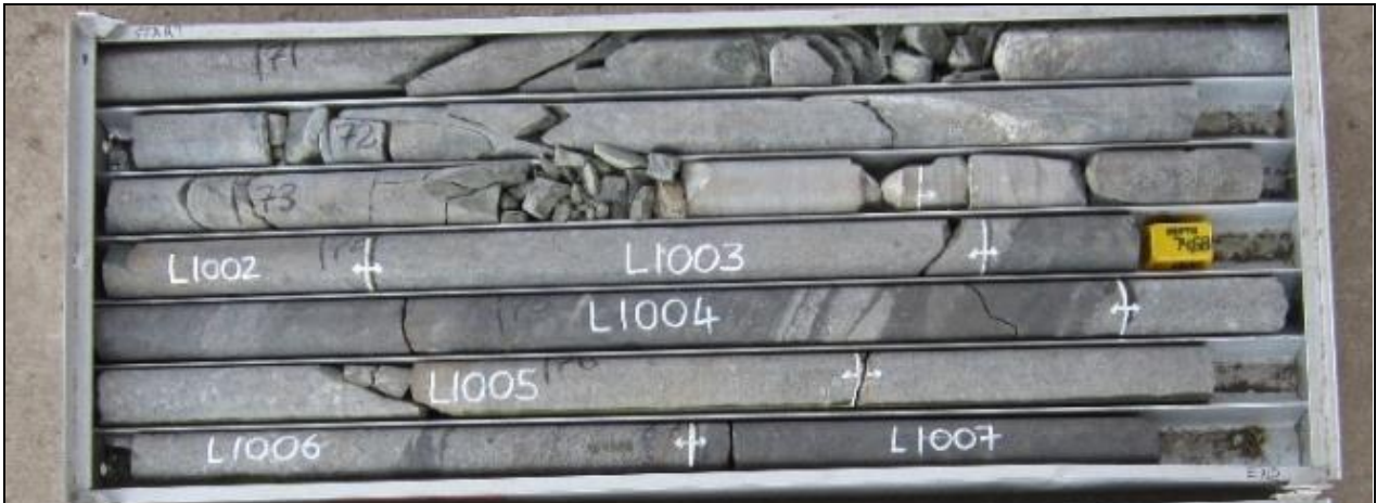
Figure 9.7 – Typical cores showing pyroxenite from the hangingwall of the LG6A
