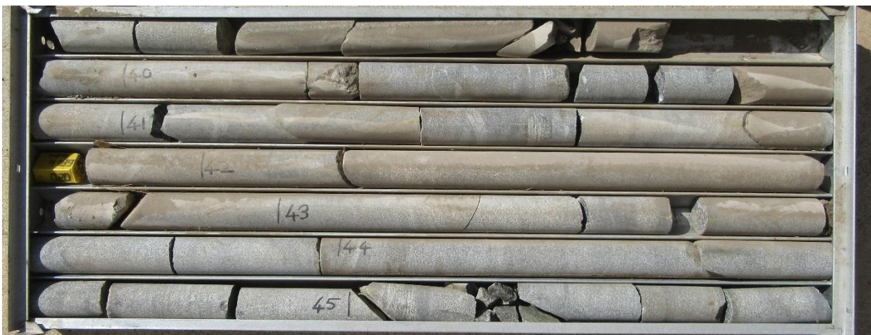
Figure 9.8 – Typical cores showing norite in the hangingwall of the MG4
