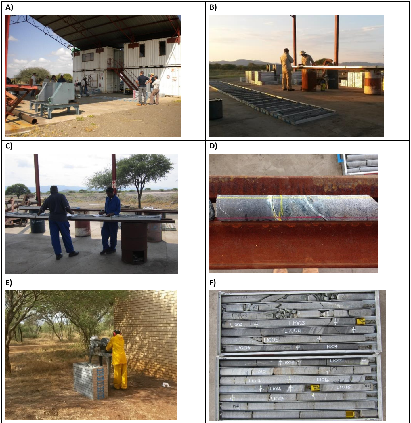
Figure 7.8 - Core processing and sampling; A) Memor Mining workshop used as the core shed; B) Core logging using tablets; C) Core processing area; D) Cut (yellow) and reference (red) lines drawn on the core; E) Core cutting; F) Samples marked with a water resistant paint marker (Source: MSA, 2015)
